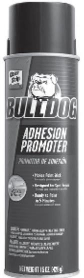
**Spot & Panel Repair:** Bulldog can be used before epoxy, urethane or polyester fillers to promote adhesion to polypropylene and TPO bumpers. Apply primers to all metal and filler areas. Sand all areas to be painted with 320 grit or finer. Apply 2 medium coats Bulldog, allowing 3-5 minutes flash between coats. Allow 5 to 10 minutes dry time before applying basecoat.
