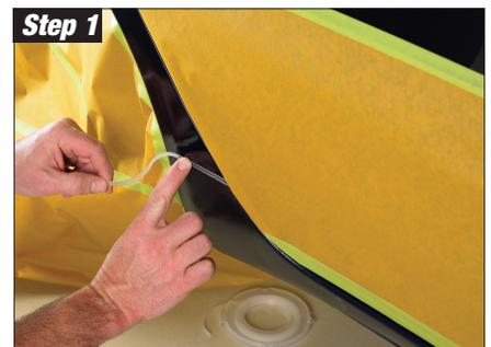
Apply tape exactly where the stone chip coating should transition. Use additional masking material above tape to protect the rest of the panel from overspray.
