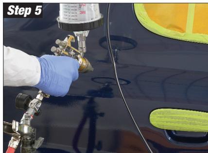
Apply initial coatings. (For sealer/color/clear application, apply sealer and one color. For color/clear application, apply all color coats.)
