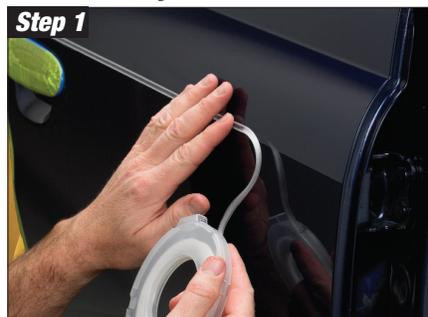
Apply tape to the body line. Use additional masking material to protect the rest of the panel from overspray.
