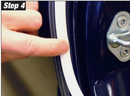
Apply additional masking material behind the strips to prevent overspray.
