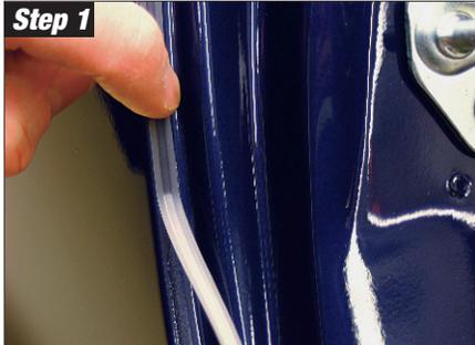
Apply the first strip, following and aligning the outside body line of the jamb with the outer edge of the tape.
