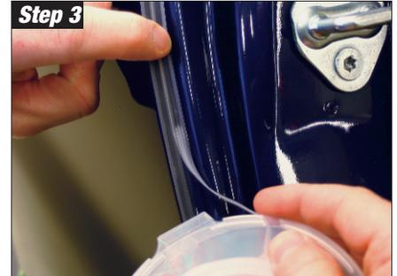
Apply a second strip of tape that overlaps the inner edge of the first strip.
