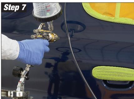
Apply the remaining coatings. Leave last strip in place until bake cycle is completed.
