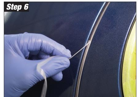
After the initial coatings have dried, grip the tab and remove the outer strip of tape. Pull tape back on itself and directly out of the jamb.
